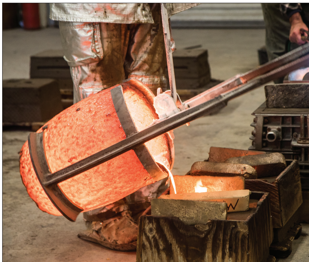
The patterns in the Rostand collection can be used to make molds, which the Foundry can then use to create parts for boat owners.
