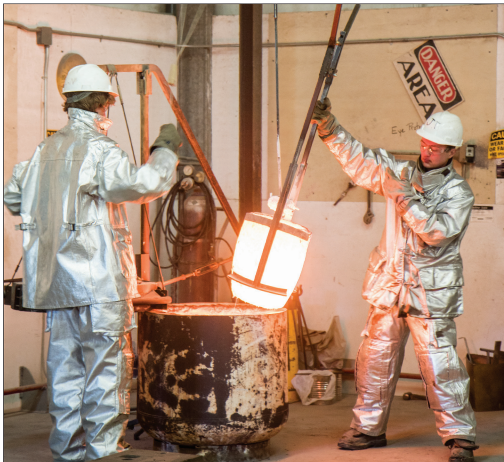
Jesse Thomas and Daniel Burgess heat up metal alloys to pour into molds and create marine parts at the Port Townsend Foundry. Leader photos by Lily Haight
