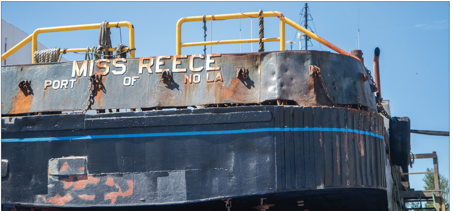
Hauled out at Port Townsend's Boat Haven, Miss Reece was transformed from an oil-industry supply shuttle to a salmon tender for the Alaska fisheries. Fuel tanks were yanked out and replaced with deep wells for storing and icing the catch. Oil service cranes came off to be replaced with fishing fleet gear and the renamed "Currentsea" was offshore in Alaska just two months after leaving the Gulf of Mexico. Leader photo by Lily Haight
